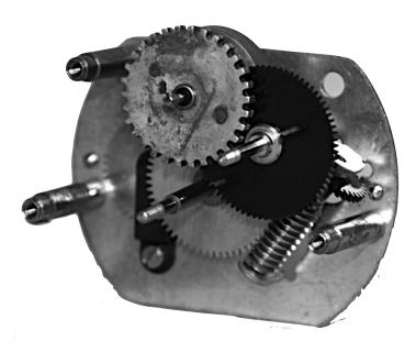
This movement is 2½ inches in diameter. Front and back plate are both brass with riveted on steel formers for the rotor magnetic field.
